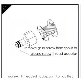
tighten firmly with allen key
