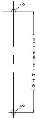
4. Drill two  $\phi$ 6mm holes according to above picture.
