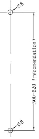
5. Mount bottom bracket on the  $\phi$ 6 hole by expansion plug and tapping screw.
