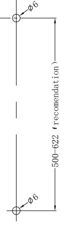
5. Mount bottom bracket on the  $\phi$ 6 hole by expansion plug and tapping screw.
