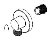
Screw elbow body on to outlet.
