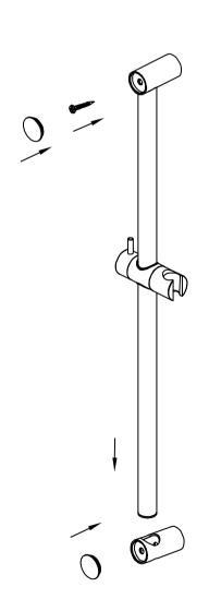
6. Plug shower rail in bottom bracket. Mount top bracket on the top hole by expansion plug and tapping screw.
