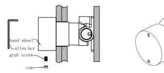
3. Make hand wheel into connecting rod, turn the hand wheel counterclockwise to the end. Then reinstall the hand wheel, make the "C" should be on twelve o'clock direction and "H" on the six o'clock direction, according to above picture. Then tighten grub screw of hand wheel by allen key, put cap into hand wheel.
