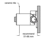
1. Fix body on nogging and ensure installation depth is 51-66mm from nogging to ceramic tile.
