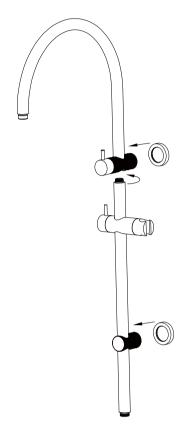
Screw shower rail into shower arm component. Tighten firmly.
