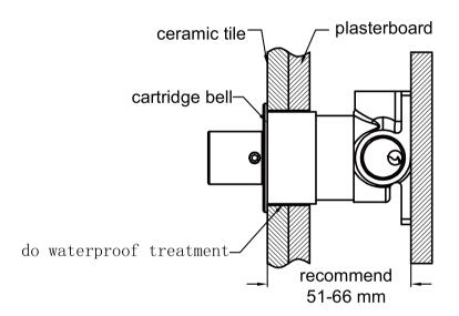
2.Put cartridge bell onto body and do waterproof treatment for the gap between cartridge bell and plasterboard and ceramic tile.
