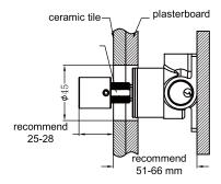
3. Adjust connecting rod and ensure depth is 25-28mm from the front of adaptor to ceramic tile.
