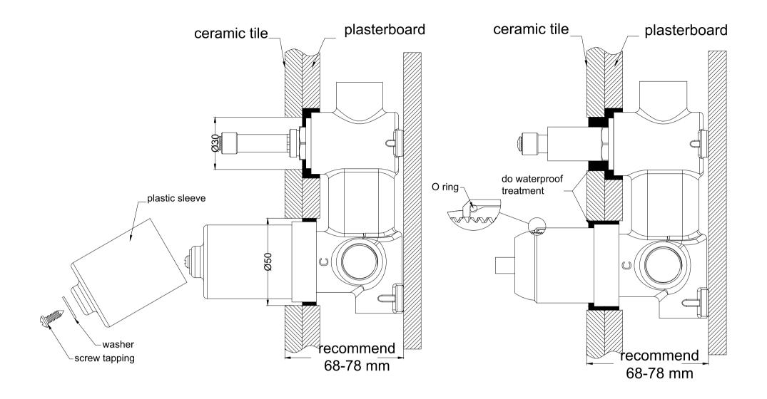
1.Drill a  $\varphi$ 50mm and a  $\varphi$ 30mm hole in the ceramic tile, then position it as shown
