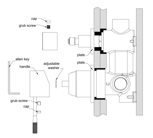
6.Slide the backplates onto body.7.Attach the washer to cartridge rod,
