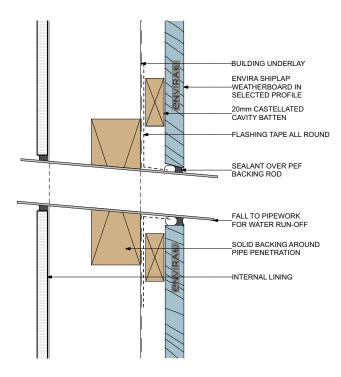
Shiplap Cavity Fix **Fascia Eaves - No Soffit 6016 2D**:
