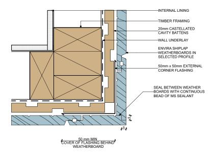
Shiplap cavity fix drawings
