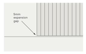
For a full run wall, ensure an allowance of 1mm expansion gap for every metre of horizontal wall covered.
