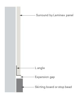
Finish your wall by installing a skirting board to the bottom of the wall, allowing room for an expansion gap. You can then fill the expansion gap with caulking to create a smooth complete look.
