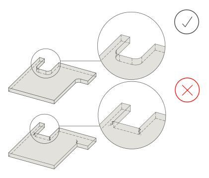
Cut-outs can be made with a router or by pre-drilling a hole with an appropriate diameter drill bit to meet internal radius requirements and then cut between drill holes.
