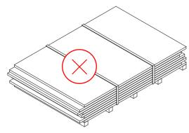
All straps and restraint devices must remain grit and burr free and suitably tensioned to prevent movement of the product when transporting. Covered loads are recommended to prevent damage during transportation.
