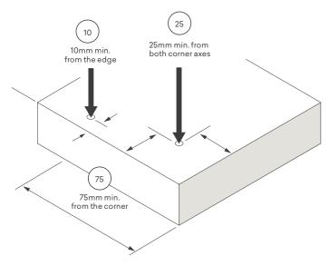
When applying fixings with power tools (nail gun, screw gun), only use enough pressure to drive the head of the nail or screw marginally below the surface of the panel. Splitting of the panel can occur if the pressure is too high or if the fixing is driven in too far and tooling marks will show on the finished surface.
