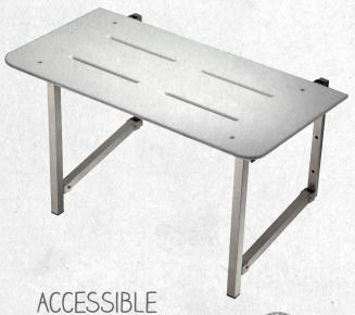
Stainless steel frame. Wall-mounted, fold down and fold up. 350kg load tested. NZS 4121:2001 compliant. Load bearing strength is dependent on wall base structure strength.
