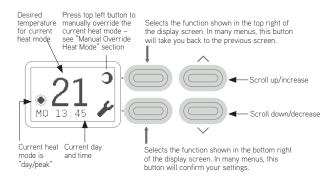
The timer has two heat modes: one for "day/peak" and one for "night/off peak". You can set a different temperature for both of these periods, for example, to keep the room warm during the day while you are using it and then to take the chill off the room when you are sleeping.
