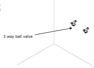
**4.** Fit the non-return valve from the installation kit into the hot 3 way ball valve, ensure that the flow arrow is the correct way (if fitted the wrong way no water will come through the valve).
