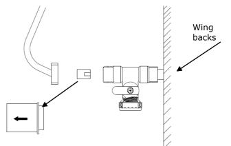
O-ring to be inserted first into the 3 way ball valve
