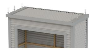
Using tinsnips, cut the side of the barge flashing flush with ridge flashing.
