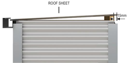
(Note: Use tek screws on lower edge of roof sheets and 50mm clouts on upper edge as this is covered by ridge flashing)
