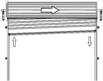
If the door rolls up crooked with the RIGHT HAND SIDE higher than the left proceed as follows:
