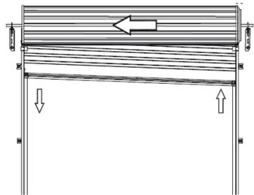
If the door rolls up crooked with the LEFT HAND SIDE higher than the left proceed as follows:
