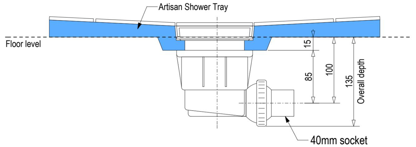
Ensure a minimum recess size of 250mm wide x 250mm long x 150mm deep for the channel drain and waste outlet
