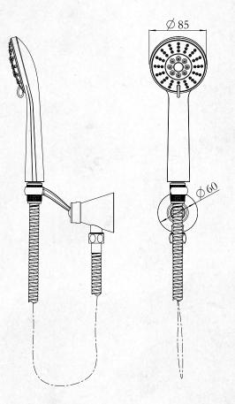
CLASSIFICATION: Suitable for Mains Pressure only INLET CONNECTIONS: 1/2 " BSP WORKING PRESSURE: 150 - 500kPa OPERATING TEMPERATURE: 5 °C - 70 °C
