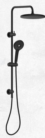
CLASSIFICATION: Suitable for Mains Pressure only INLET CONNECTIONS: 1/2 " BSP WORKING PRESSURE: 150 - 500kPa OPERATING TEMPERATURE: 5 °C - 70 °C
