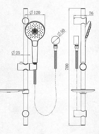
CLASSIFICATION: Suitable for Mains Pressure only INLET CONNECTIONS: 1/2 "BSP WORKING PRESSURE: 150 - 500kPa OPERATING TEMPERATURE: 5 °C - 70 °C
