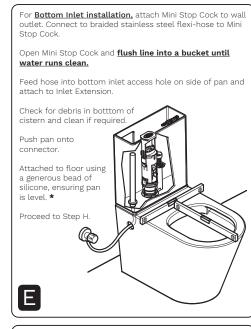
Connect Mini Stop Cock to braided stainless steel flexi-hose and **flush line into a bucket until water runs clean.**
