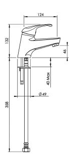
CONSTRUCTION: Brass body CARTRIDGE TYPE: Ceramic CLASSIFICATION: Suitable for all pressures INLET CONNECTIONS: 1/2 " BSP WORKING PRESSURE: 35 - 500kPa DIMENSIONS FOR FITTING: 35mm diameter hole OPERATING TEMPERATURE: 5 °C - 65 °C
