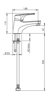
CONSTRUCTION: Brass CARTRIDGE TYPE: Ceramic (SP033550) CLASSIFICATION: Suitable for all pressure systems INLET CONNECTIONS: 1/2 " BSP Female (male nipples provided) WORKING PRESSURE: 35 - 500kPa DIMENSIONS FOR FITTING: 35mm diameter hole required OPERATING TEMPERATURE: 5 °C - 80 °C WATER FLOW RATE: 8.0 l/m (mains pressure) - 8.5 l/m (low pressure)
