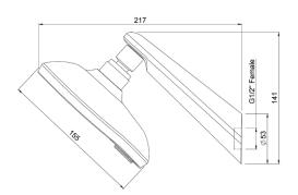
CONSTRUCTION: Brass arm CLASSIFICATION: Suitable for all pressure systems INLET CONNECTIONS: 1/2 " BSP Female WORKING PRESSURE: 35 - 500kPa OPERATING TEMPERATURE: 5 °C - 70 °C
