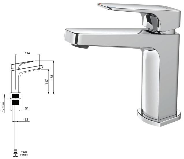
**CONSTRUCTION:** Brass body **CARTRIDGE:** Ceramic
