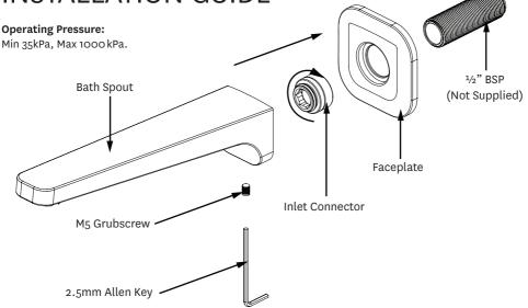
NOTE: Maximum hole diameter through wall for ½" BSP tube is 22mm.
