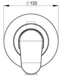
CONSTRUCTION: Brass body CARTRIDGE TYPE: Ceramic (SP033510) CLASSIFICATION: Suitable for mains pressure only INLET CONNECTIONS: 1/2 " BSP WORKING PRESSURE: 150 - 1000kPa DIMENSIONS FOR FITTING: OPERATING TEMPERATURE: 5 °C - 80 °C
