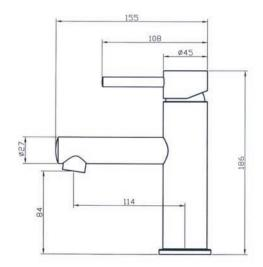
**CONSTRUCTION:** Brass body **CARTRIDGE TYPE:** Ceramic
