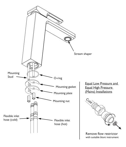
All pipework must be thoroughly flushed prior to the installation of the mixer. Inline filters must be fitted on both hot and cold supplies to prevent foreign particles damaging the ceramic cartridge.
