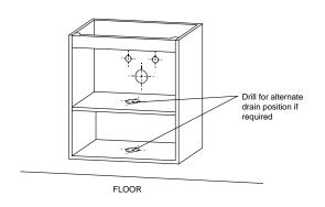
(C) With a suitably sized hole saw drill the holes for the water supply and waste.
