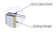
Glass To Wall Tolerance DETAIL A
