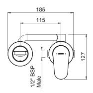
**CONSTRUCTION:** Eco Brass **CARTRIDGE TYPE:** Ceramic
