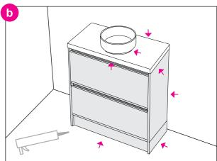
When sealing a vessel or semi inset basin it is important to put a bead of silicone around the edge where the basin meets the top. As well as where the top meets the wall.
