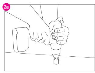
Firmly clamp top down before drilling (handle with care to ensure no damage occurs to the top during this process)
