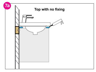
Position the top so that it has an equal amount of overhang on each side and use a level to ensure the vanity top surface is level. Note: If the vanity is being installed in a corner, a packing strip is required and basin location will vary.
