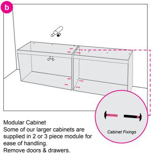
Use cabinet connectors supplied to join cabinets in pre-drilled locations.
