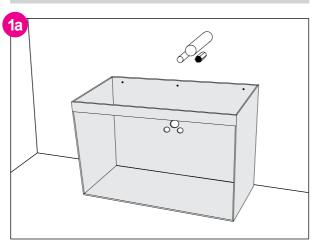
Remove doors & drawers and drill holes for plumbing in the back panel and/or base of the cabinet with an appropriate sized hole saw. Pre-drill screw locations for fastening to wall in step 4
