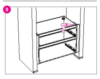
Secure your spacers using pilot holes, drilled in Step 3, and screws provided.
