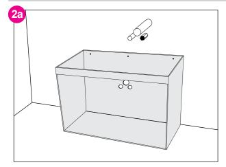
Remove doors & drawers and drill holes for plumbing in the back panel and/or base of the cabinet with an appropriate sized hole saw. Pre-drill screw locations for fastening to wall in step 6.
