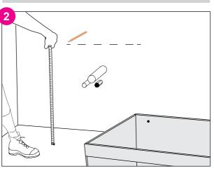
Mark the position of the top of the vanity - factor in the top/ basin thickness to get the correct height.
