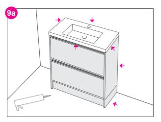
Apply silicone on the seam between the edge of the vanity top and the wall, smooth the bead, and allow to cure before use. Materials used for the construction of this unit are water resistant and not waterproof. A bead of sealant (specifically formulated for bathrooms) must be used to seal edges where water penetration can occur i.e. Between the basin and the cabinet and between the wall and the floor.
