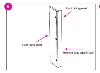
Assemble spacers by locating cam pins into cams. Secure by locking cams into lock position. Front facing panels trimmed edges are positioned against wall.
