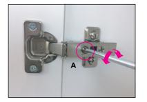
To move doors sideways or to level each door - turn screw **A** Clockwise or Anti Clockwise
