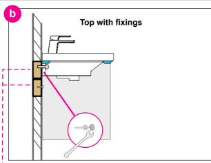
3. If installing a basin with bolt fixings - ensure basin is fixed into nogs with supplied fixings as well as using a silicone sealant to the top of the cabinet.
