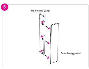
Screw cam dowls into trimmed outward facing panel. Knock cams into rear fixing panel.
