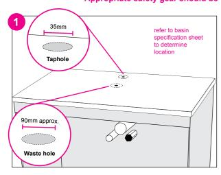
Decide on the location of your taphole & basin waste hole and measure out position. Drill a pilot hole through the counter top at your center point. This hole should be just slightly smaller than the size of the pilot bit of your hole saw.
