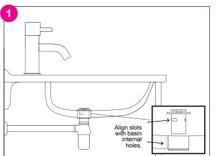
When fitting waste to basin do not overtighten or the basin may be damaged. Use suitable overflow waste and align the slots with the internal holes in the basin. Ensure that no excess silicone or putty is obstructing the water flow.
