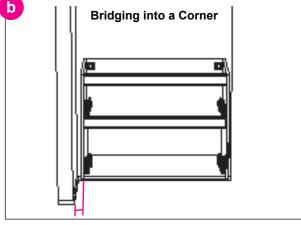
Measure gap to determine spacer width.
