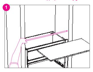
Measure front & back lengths to determine measurements for the perfect fit.
