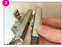
To re-install insert tongue and hooks into cut out, gently pull forward and press rear back into position.
