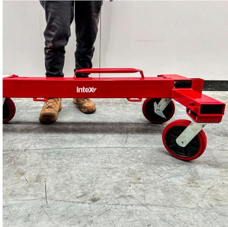
6. With the arms stowed and locked in the storage and transport position, the cart can be conveniently handled for compact transportation.
