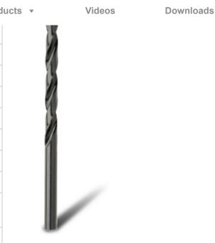
BLACK FINISH (also called blue finish) A black finish is achieved by steam tempering, a thermal process resulting in a porous tool coating. This surface helps to keep lubricant on the tool, particularly important on the cutting edges, thus reducing friction and cold welding. The result is increased tool life. Black finish tools are generally recommended for ferrous applications where the oxide layer aids chip flow and heat dissipation.
