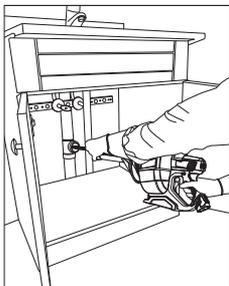
**NOTE:** To avoid fatigue or to free a hand for easier cable feeding, the tool can be placed on the flat tool base during use.
