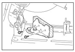
When the cut-off wheel has worn down, raise the cutting position by putting a spacer block which is slightly narrower than the workpiece as shown in the figure. This will help you to utilize the wheel economically.
