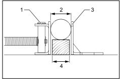
1. Vise plate 2. Workpiece diameter 3. Guide plate
