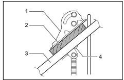
1. Guide plate 2. Spacer block (over 190 mm long x45 mm wide) 3. Workpiece (over 85 mm wide)
