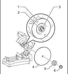
Inner flange 2. Ring 3. O-ring 4. Cut-off wheel
