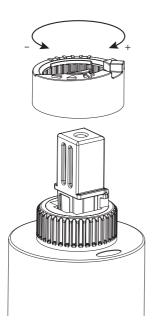
Turn the temperature limiting ring clockwise (+) to increase maximum hot temperature, anti-clockwise (-) to reduce the maximum hot temperature.
