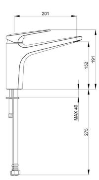
**CONSTRUCTION:** Brass body CARTRIDGE: Ceramic CLASSIFICATION: Suitable for all pressure systems **INLET CONNECTIONS:** 1/2 " BSP Female WORKING PRESSURE: 35 - 1000kPa DIMENSIONS FOR FITTING: 35 - 38mm diameter hole OPERATING TEMPERATURE: 5 °C - 80 °C WATERFLOW RATE: 6.5 l/m
