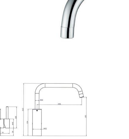
CONSTRUCTION: Brass body CARTRIDGE TYPE: Ceramic (SP033570) CLASSIFICATION: Suitable for mains pressure only INLET CONNECTIONS: 1/2 " BSP Female WORKING PRESSURE: 150 - 1000kPa DIMENSIONS FOR FITTING: 35 mm diameter hole OPERATING TEMPERATURE: 5 °C - 80 °C
