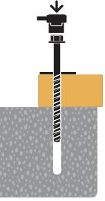
Install with either a socket or cordless impact driver. Apply pressure against the fixing and rotate to engage the first thread. Continue to tighten the anchor until flanged head is firmly seated against fixture.
