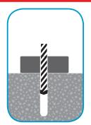
With the correct diameter drill bit, drill a hole to the correct depth. (see general information section of this document).
