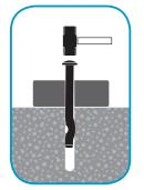
Tap in anchor until seated and flush with surface of base material.
