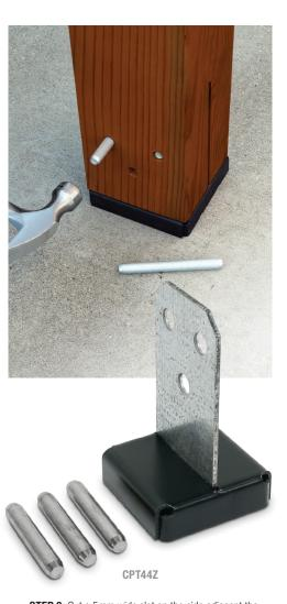
STEP 3: Cut a 5mm wide slot on the side adjacent the drilled holes. Check that the knife plate slides freely.
