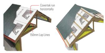
Covertek 401 can be direct fix or cavity fix and must be installed in a manner that prevents ponding of water and span no more than 1200mm.
