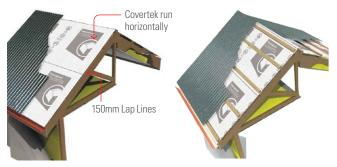
Covertek 405 can be direct fix or cavity fix and must be installed in a manner that prevents ponding of water and span no more than 1200mm.
