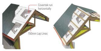
Covertek 403 can be direct fix or cavity fix and must be installed in a manner that prevents ponding of water and span no more than 1200mm.
