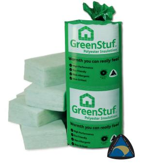
**Moisture:** GreenStuf® is not affected by moisture. Exposure to an atmosphere of 50°C at 90% relative humidity for four days showed moisture absorption by weight of less than 0.03%.
