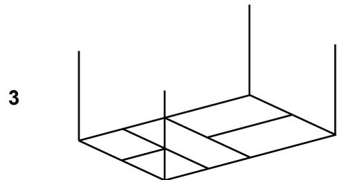
**Step 4:** Position the back wall frame on top of plates. While someone supports frame, nail in place.
