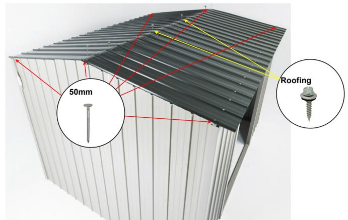
**Step 4:** Centralize Roof at the other end and nail through Rib into the Ridge Beam and Top Plates, using 50mm Clouts. Ensure Ridge Beam is straight, then Screw one 50mm Roofing Screw into Ridge Beam through each Rib on overlap (one screw per sheet). At the back, set up a String Line in centre of Top Plate. Ensure Top Plate is straight and screw, using one 50mm Roofing Screw per Rib. Repeat at the front.
