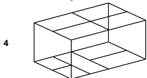
**Step 5:** Carefully roll frame over onto its base. (Pieces of timber from the packaging may be used to temporarily brace the frame before rolling it over). Position 1.625 End Wall Nogs .883m down from Top Plate and nail in place. If fitting a Kiwi Floor, fit Floor Joists now. Space joists equally and nail in place using three 75mm nails per end.
