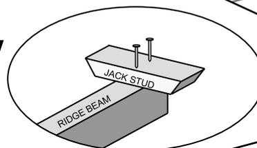
**Step 6:** Position a Jack Stud on each end of Ridge Beam and nail in place using two 75mm nails each end (**fig. 1**). Turnover Ridge Beam / Jack Studs, position centrally on 1.715m Top Plates and nail to Top Plates using two 75mm nails per Jack Stud.
