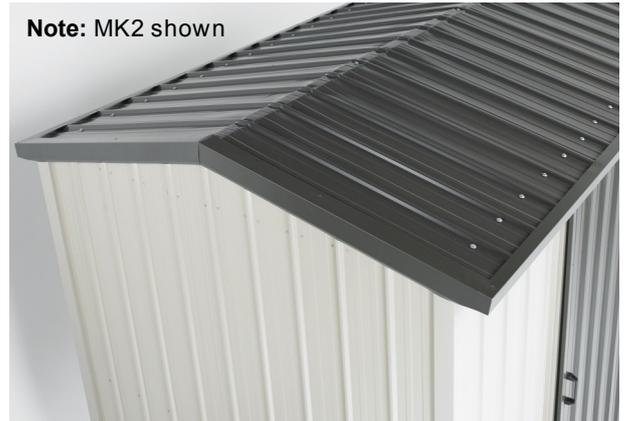
**Step 1:** Position Barge Flashing (102) on gable ends. Position a Spouting (A103) and rivet to the Barge Flashing at each end. Repeat with other Spouting.
