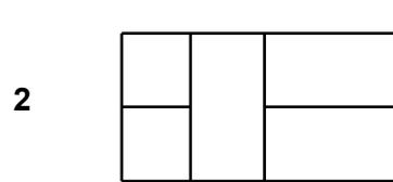
**Step 3:** Select two 1.715m Base Plates (Green) and two 1.715m Top Plates (Red). With front wall lying on the ground, nail Plates to frame. Ensure Green joins to Green and Red joins to Red.
