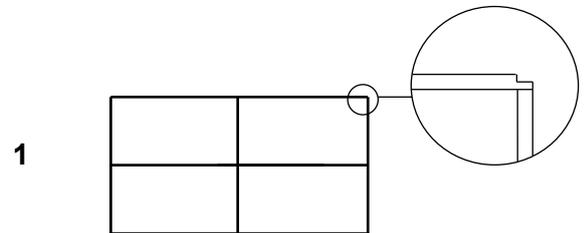
**Step 2: Front Wall:** Select one 3.380 Base Plate (Green), one 3.380m Top Plate (Red), four Studs (Yellow), one .785m Nog and one 1.622m Nog. Nail studs to each end of Plates. Nail in remaining two studs using Nogs to get correct position. Position Nogs .883m down from Top Plate and nail in place.
