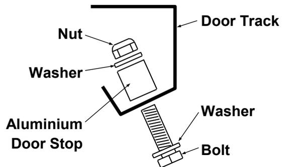
**Step 4:** Clean out ALL drill filings. Also make sure the Wheels are cleaned of drill filings. Re-hang Door, then insert door stops into the pre drilled holes at end of tracks as shown in diagram. Tighten with two spanners
