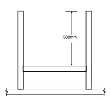
Step 1: Lay out the two window studs (883mm) and Nog (634mm) on a flat surface. Position Nog and nail in place using 2x 75mm nails at each end.
