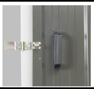
Using six rivets and one 50mm clout attach hasp to Door Jamb Flashing and the staple to the Door as shown.
