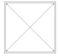
**Step 8:** Temporarily brace each side and roof, making sure each side is square. Nail strip bracing to outside of Frame (see page 4), making sure it is tight. Nail multigrip brackets to each of the four bottom corners (two per corner). Use 30mm bracket nails supplied.
