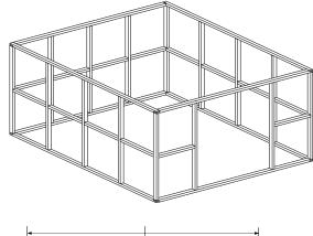
Step 5: Position middle Jack Stud, centrally on End Wall Top Plates and nail in place. Nail remaining Jack Studs in. Position middle Ridge Beam to Jack Stud and skew-nail in place using two 75mm nails each end. Pre-drilling holes before nailing will prevent timber from splitting.
