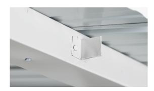
Step 2: Position right hand Door Track (D107) on front wall up against underside of Roof, with left hand end hard against the Centre Door Stop. Pre-drill hole in centre and rivet in place. Remove ALL drill filings
