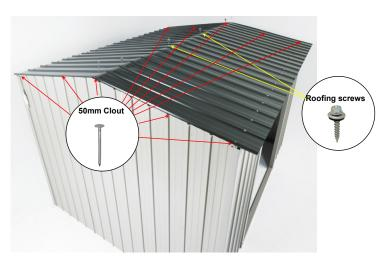
Step 2: Starting from the left hand end, centralize Roof on Ridge Beam. Ensure Roof is tight against end Wall Sheets, predrill then nail one 50mm Clout through Rib into the Ridge Beam. At the back, line up Ribs on the Roof Sheet with the Ribs on Wall Sheet. Using one 50mm Clout, nail through Rib into Back Top Plate. Repeat at the front.
