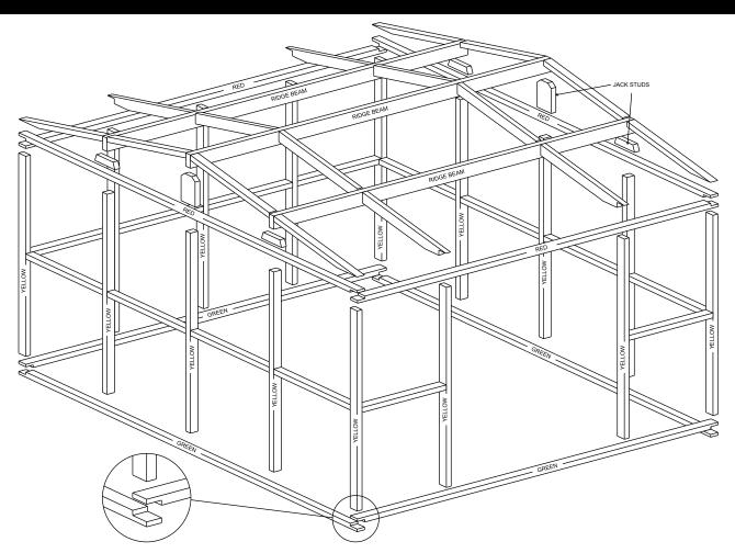
Note: For sheds with the Raised Floor Modification option the studs will be 1.780m long to allow the Wall Sheets to protrude 20mm below the Bottom Plate. Refer to Raised Floor Modification section (Page 15).
