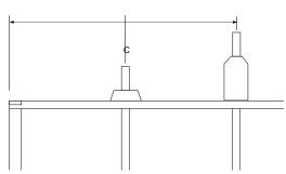
**Step 6:** Place intermediate Roof Beams by using Roofing Nogs to determine correct position (see *fig. 2*). Nail intermediate Roof Beams in place. Nail 70 x 45mm Roofing Nogs in place (End Wall) and 90 x 45mm Roofing Nogs in place (Middle).
